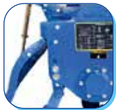
ADJUSTABLE TRAILING BOARD AND DEPTH SKID
