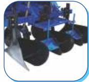
FURROW OPENER WITH REPLACEABLE WEAR & TEAR POINT AND DEPTH ADJUSTABLE SPIKE
