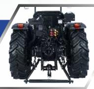
This tractor's hydraulic system is built for heavy-duty operations. Equipped with CAT II three-point linkage and an impressive 2500 kg lift capacity, it ensures smooth, precise control and allows you to tackle any job with ease. A high flow rate of 45 LPM combined with 90% hydraulic pump efficiency ensures smooth, precise control.
